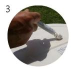
Cut the applicator nozzle from its base and apply the entire contents of flexible polymer adhesive in the center of the back, without spreading. Only one applicator content is required.
